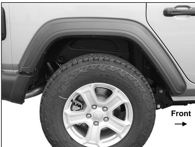
(Fig 1) Release clips and all hardware attaching inner fender liner to outer fender
