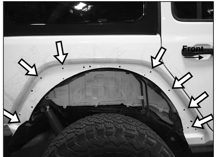
(Fig 4) Drill 7/16 hole in body panel at (7) locations (arrows). NOTE: These locations are not accessible from back of body panel
