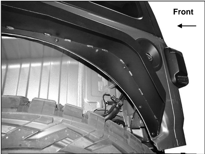
(Fig 13) Attach rear of Fender to mounting locations on body, (driver/left Fender pictured)
