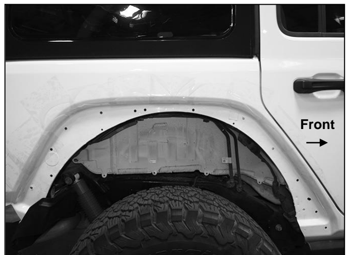
(Fig 2) Firmly pull fender straight out from vehicle. Remove any clips still attached to body
